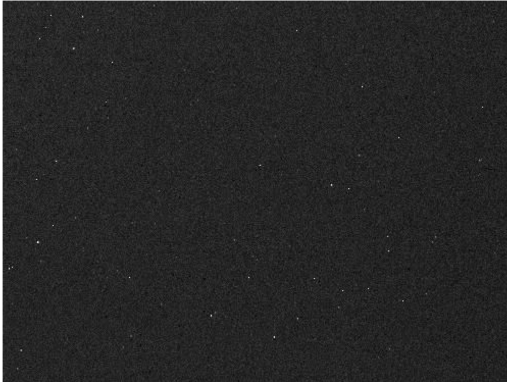
Fig. 2 Accumulation of dark current on CCD (small area of 30 min. dark frame brightened 37 times for ease of viewing).
